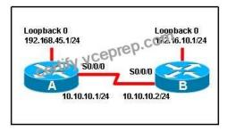
When running OSPF, what would cause router A not to form an adjacency with router B?
