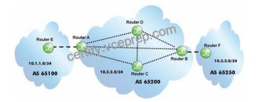
After router A receives the BGP update for the 10.3.3.0/24 prefix, which routers will the route be propagated to?
